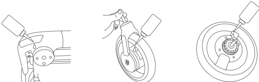
Besides that, there are eight ball bearings in the stroller (2 in each wheel), which should be greased regularly and protected from dirt and liquids. In the event that such substances get in, the ball bearings should be cleaned, dried and greased with several oil drops. Any spillage of the oil should be wiped with a dry cloth.
